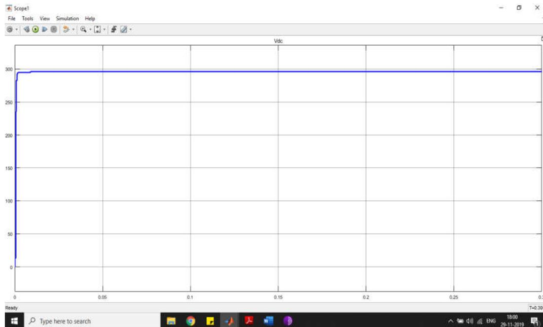
Figure 10: DC-DC Isolated Converter Output Voltage
