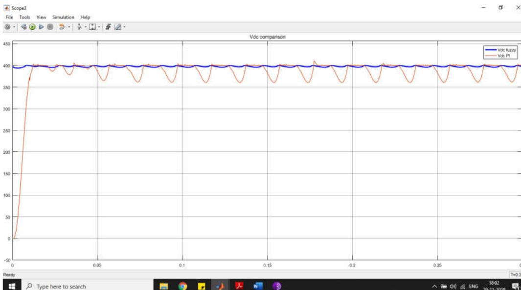
Figure 12: Output Voltage Comparison of Landsman PFC Converter with PI and Fuzzy
