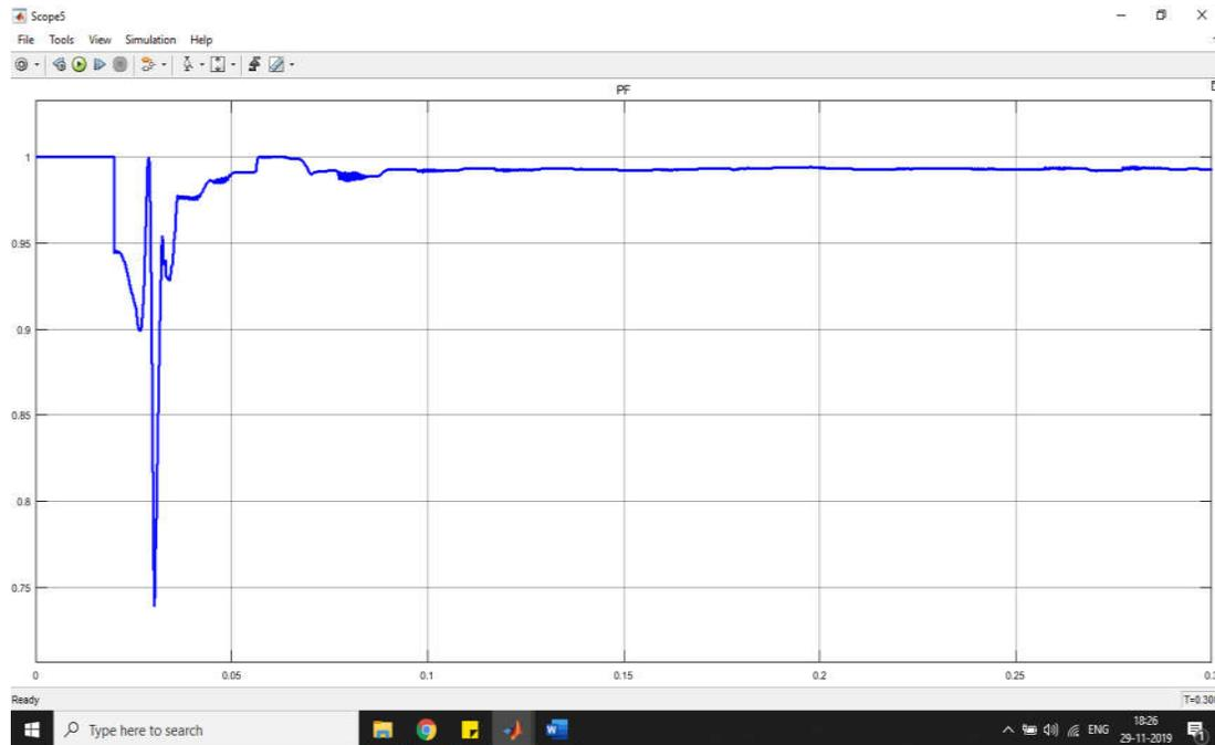
Figure 7: Power Factor of Source with PI Controller
