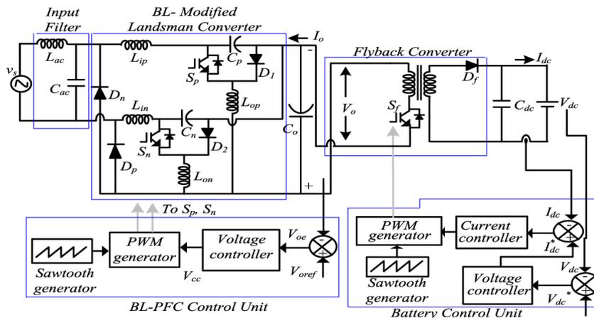
Figure 3: Modified Bridgeless Landsman Converter
