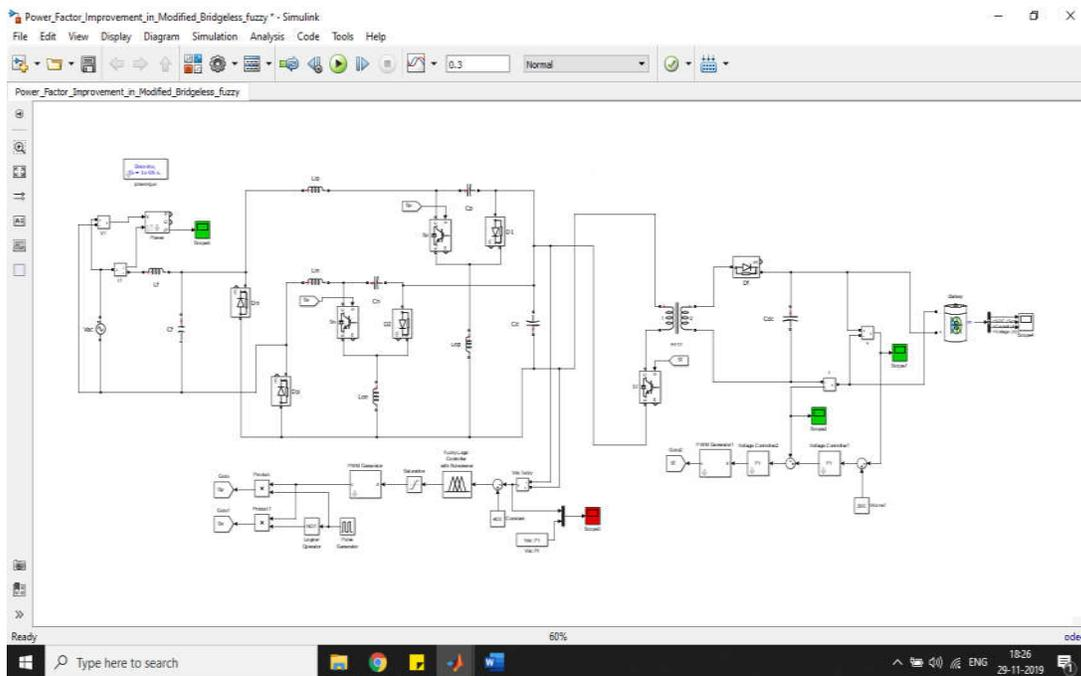
Figure 6: Modeling of Proposed Topology with Fuzzy Interface System
