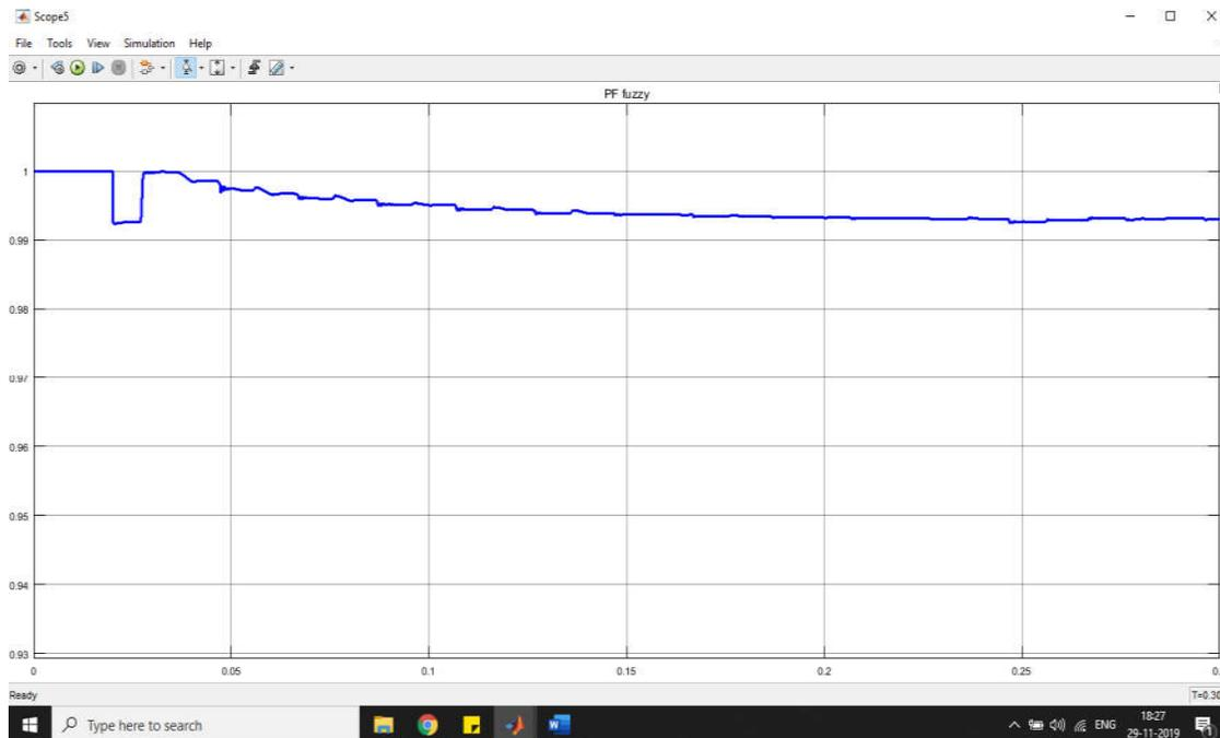
Figure 8: Power Factor of Source with Fuzzy Controller
