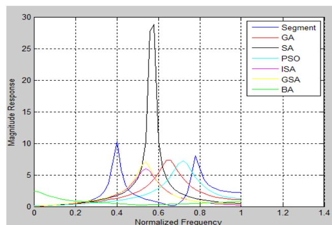
**Figure 4. Comparison of Magnitude Response of 4<sup>th</sup>-order IIR-DDs using different optimization algorithms**
