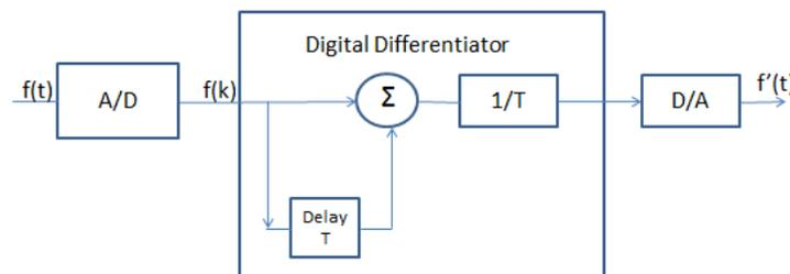
Figure 1. Block Diagram of Digital Differentiator
