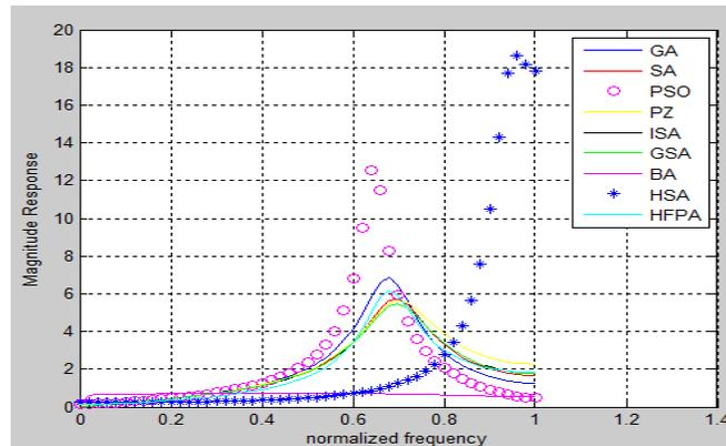
**Figure 2. Comparison of Magnitude Response of 2<sup>nd</sup>-order IIR-DDs using different optimization algorithms**
