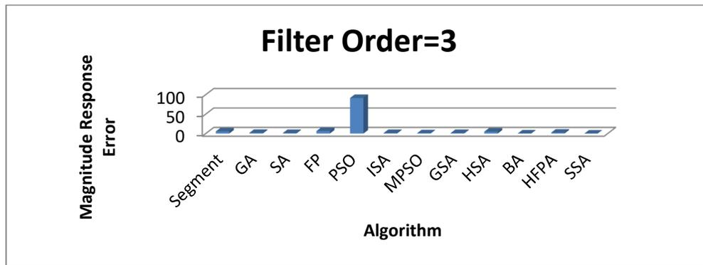
Figure 6. Comparison of magnitude response error of 3<sup>rd</sup>-order digital differentiators using different algorithms
