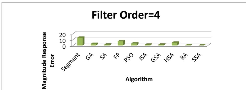
Figure 7. Comparison of magnitude response error of 4<sup>th</sup>-order digital differentiators using different algorithms
