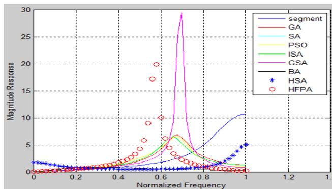
**Figure 3. Comparison of Magnitude Response of 3<sup>rd</sup>-order IIR-DDs using different optimization algorithms**
