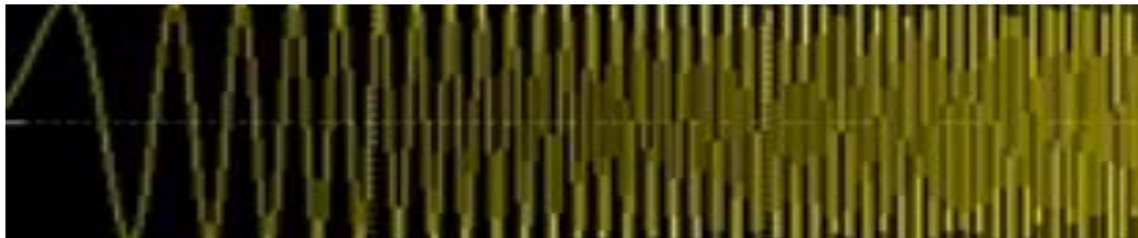
Fig.3 The DDS generated Chirp (LFM) signal
