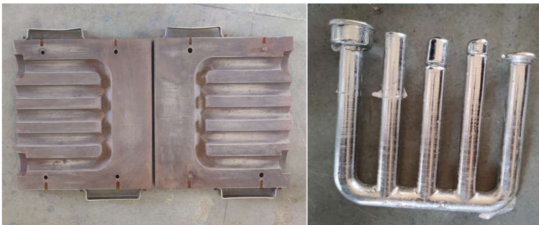
Fig.2 (a) Metallic Die (b) Casting after solidification
