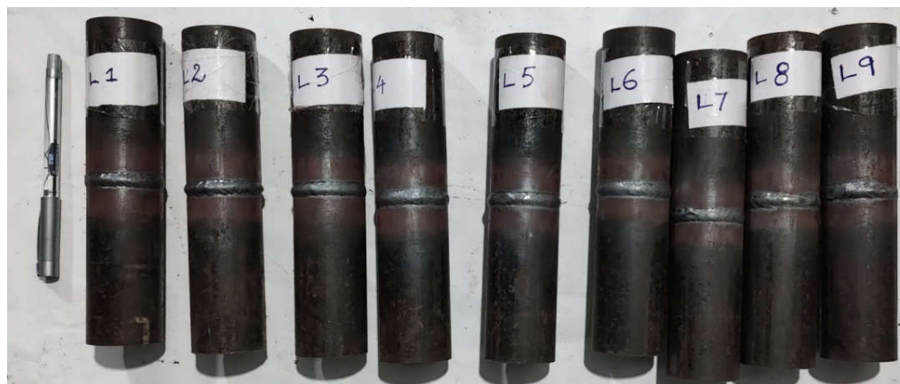
Figure 2. 2.25 Cr 1 Mo steel pipe joints
